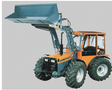
Figure 4.41 Tractor with “center-steering”
