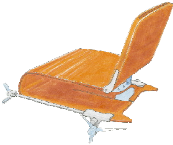
Design of the slider, the backrest folding mechanism, and the overall shape of the chair
