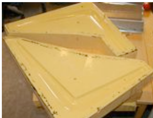
Figure 7.12 Moulds for side parts
