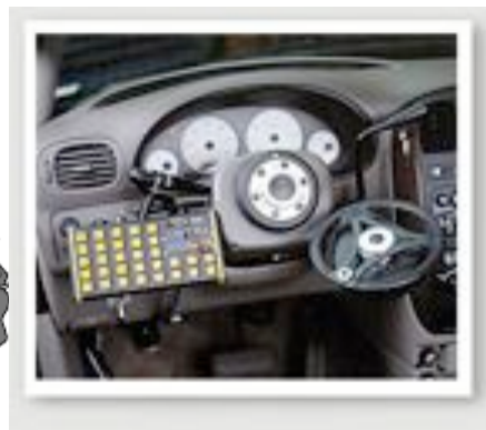
Figure 4.11 Miniature and original steering wheel with control panel
