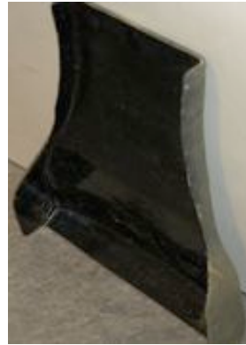
Figure 7.14 Mould for backrest
