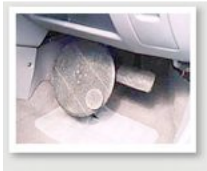
Figure 4.12 Foot steering device
