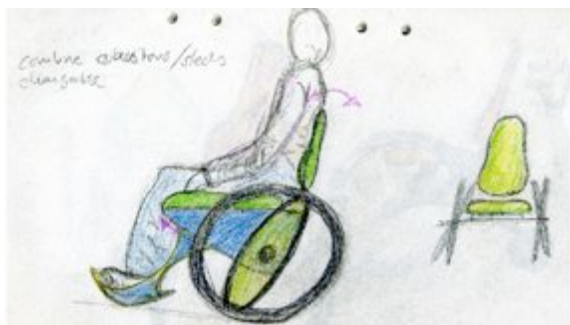
56. Combined saucer caster/camber angle change
