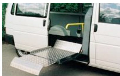
Figure 4.14 Visualization of a wheelchair lift form U-lift.
