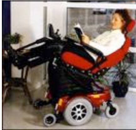
Figure 4.2 Maneuverable power chair with adjustable seat and device for not tipping over.
